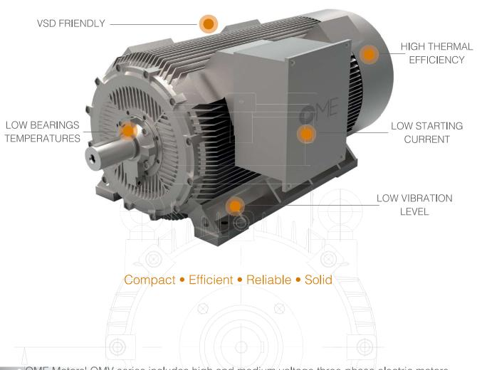
OME Motors' OMV series includes high and medium voltage three-phase electric motors characterized by a compact structure and IC 411 cooling system. These are self-ventilating motors using a special fan connected to the shaft: cooling air is external and touches the surface of the casing.
