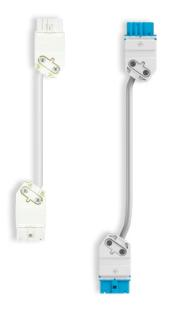
The extensions for mains and internal bus for the flat surface-mounted module system for decentralized installation, which can be mounted on a mounting rail, may have a maximum length of one meter in the system. It locks automatically upon plugging. The mechanical coding means that the mains connection cannot be confused with the bus connection.
