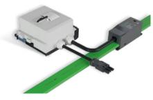
The RCB/MCB combination with the flat cable tap-offs for the Wieland 10 mm<sup>2</sup> flat cable is used for decentralized fusing and is integrated in the flat surface mounted housing which can be fitted on DIN rails for decentralized installation. It can be mechanically linked to the gesis® FLEX system and forwards the gesis® FLEX bus and mains wiring to the following module. The fused tap-off is pluggable in accordance with IEC 61535.
