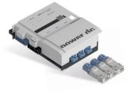
The 24 VDC; 30W power supply unit with flat surface mounted housing which can be fitted on DIN rails for decentralized installation can be added to the system. It receives mains from the upstream module and forwards mains and bus supply to the following modules. The output is wired parallel to three 2-pole connectors.
